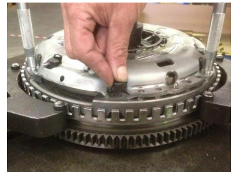
Pic 8 (screw in cover to flywheel bolts)
