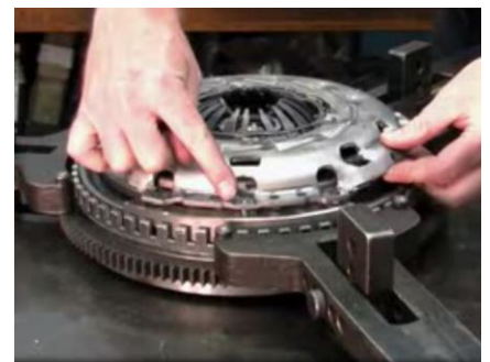
Pic 3 (pressure plate aligned with dowels)
