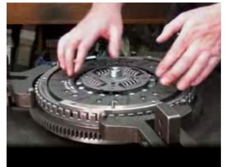
Pic 2 (driven plate over aligning tool)
