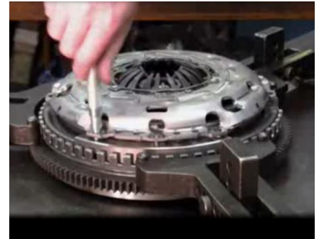
Pic 4 (fix threaded bolts until finger tight)
