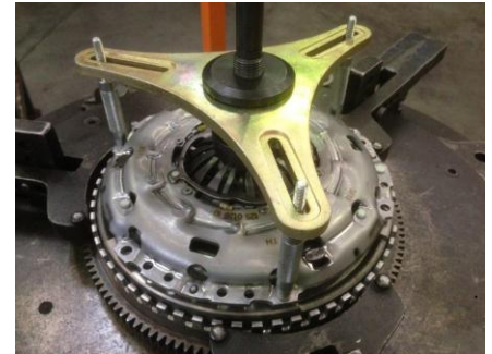
Pic 5 (clamping tool placed over assembly)
