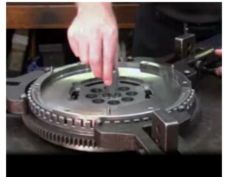
Pic 1 (locating the aligning tool)
