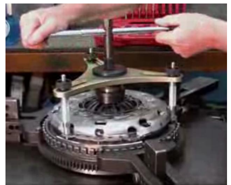
Pic 9 (rotate strut anti-clockwise to remove tool)
