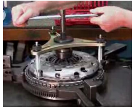
Pic 7 (rotate strut in clockwise direction)
