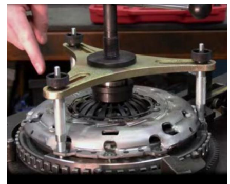
Pic 6 (secure clamping tool by using knurled nuts)
