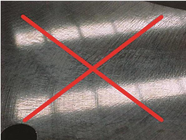
**Fig: 4.** "This flywheel has been machined with a polish finish which may promote clutch shudder".
